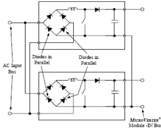
Figure 24e Connecting multiple PFCs to the AC input bus and the MICROVERTER<sup>®</sup> -IN bus parallels the lower diodes in the rectifier bridges.
